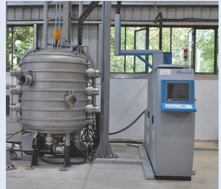
Plasma Nitriding Furnace
