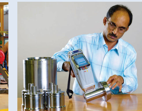
Positive Material Identification of special alloys
