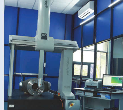
Verification of geometrical tolerances and 3D profile using Coordinate Measurement Machine
