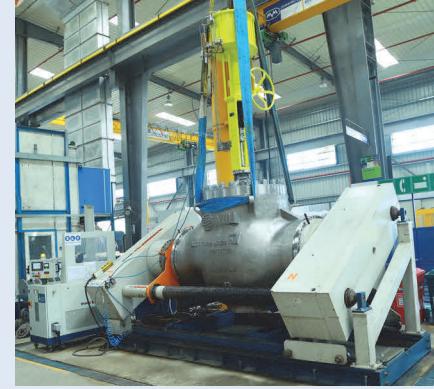
A 32 inch size valve being tested on the High pressure test bench
