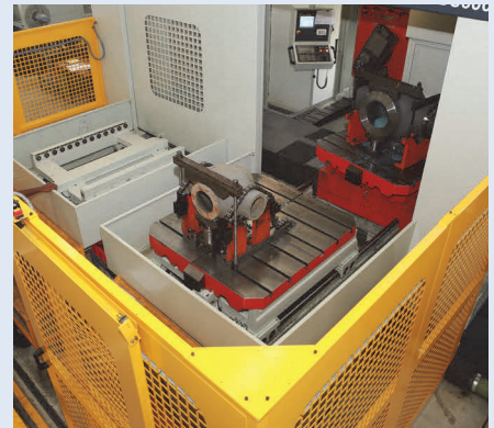
Horizontal machining centre - Valve body machining in single setting
