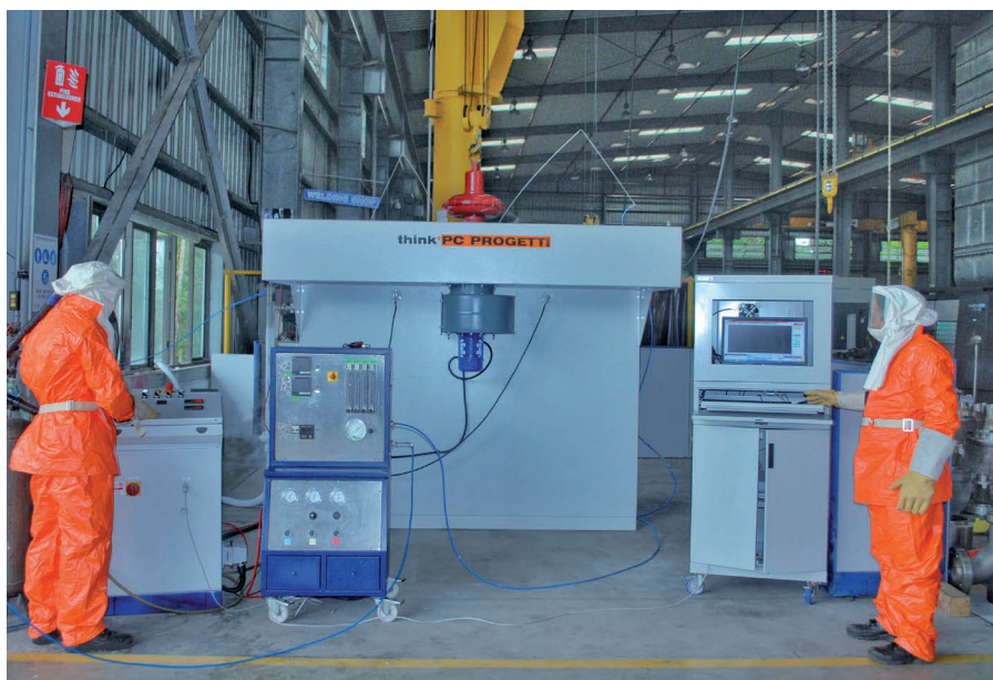
Cryogenic testing of valves with liquid Nitrogen at -196^{\circ}\text{C}
