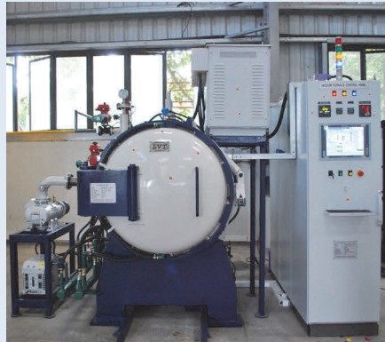
Vacuum Heat Treatment facility
