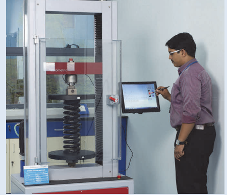
Load and deflection testing of Actuator springs
